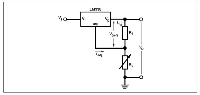
Since the 50µA current from the adjustment terminal represents an error term, the LM338 was designed to minimize Iadi and make it very constant with line and load changes. To do this, all quiescent operating current is returned to the output establishing a minimum load current requirement. If there is insufficient load on the output, the output will rise.
