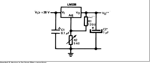
Needed if device is far from filter capacitors. \* Optional-improves transient response. Output capacitors in the range of 1mF to 100mF of aluminium or tantalum electrolytic are commonly used to provide improved output impedance and rejection of transients
