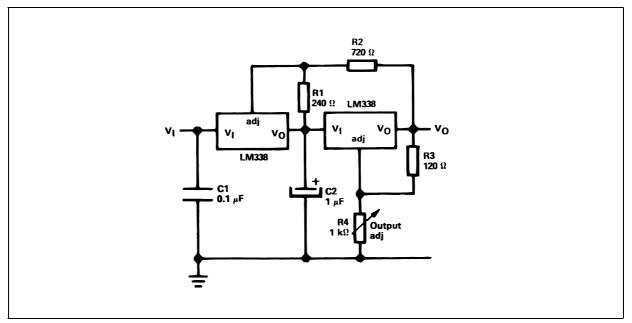
$^{*}$  R\_1 = 240  $\Omega$  for LM138 or LM238  $^{*}$  R\_2 = 720  $\Omega$  for LM138 or LM238  $^{*}$  \* Minimum output = 1.2V
