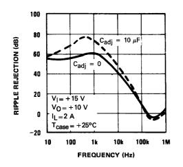
Figure 12 : Ripple Rejection
