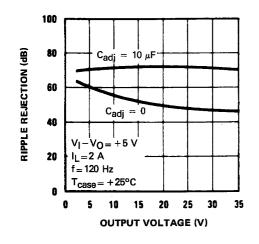
Figure 11 : Ripple Rejection
