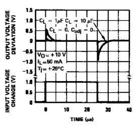
Figure 14 : Load Transient Response
