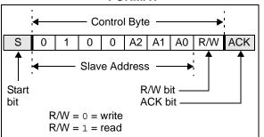
FIGURE 1-3: SPI™ CONTROL BYTE FORMAT
