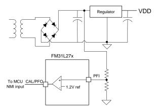
Figure 5. Comparator as Early Power-Fail Warning
