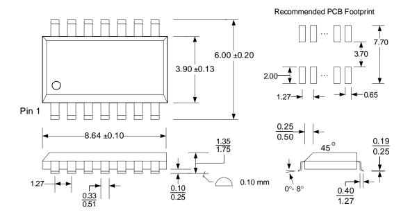
Refer to JEDEC MS-012 for complete dimensions and notes. All dimensions in millimeters.
