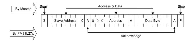
Figure 17. Byte Register Write
