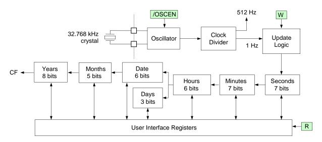
Figure 7. Real-Time Clock Core Block Diagram
