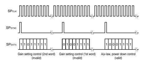
**Remark** Because gain setting control (2nd word) is input before gain setting control (1st word), gain setting control (1st word) becomes invalid. Then, because A/µ-law, power down control is input even if gain setting control (1st word) is input, gain setting control (1st word) becomes invalid.
