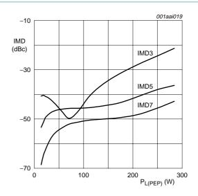
$V_{DS} = 32 \text{ V}; I_{Dq} = 1600 \text{ mA}; f_1 = 1880 \text{ MHz}; f_2 = 1880.1 \text{ MHz}.$
