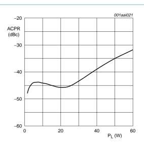
$V_{DS} = 32 \text{ V; } I_{Dq} = 1600 \text{ mA; } f_1 = 1872.5 \text{ MHz; } f_2 = 1877.5 \text{ MHz; } \text{carrier spacing 5 MHz.}$
