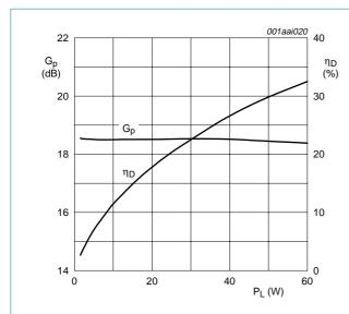
$V_{DS} = 32 \text{ V}; I_{Dq} = 1600 \text{ mA}; f_1 = 1872.5 \text{ MHz}; f_2 = 1877.5 \text{ MHz}; carrier spacing 5 \text{ MHz}.$
