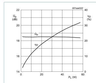
$V_{DS} = 32 \text{ V; } I_{Dq} = 1600 \text{ mA; } f_1 = 1867.5 \text{ MHz; } f_2 = 1877.5 \text{ MHz; } carrier spacing 10 \text{ MHz.}$
