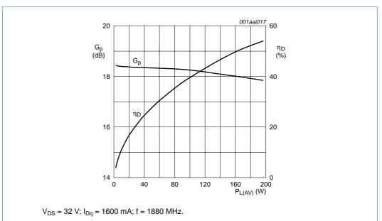
Fig 1. One-tone CW power gain and drain efficiency as function of average load power; typical values
