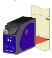
Position the background in front of the sensor light spot and press BKGD push-button. The sensor detects the mark alternating the red, green and blue emissions. Avoid background movements during this phase.
