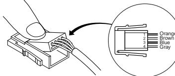
**Note 1:** Do not allow the cable to protrude from the other end of the connector cover.
