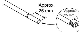
**Note:** It is not necessary to remove the sheath of the core wire.
