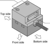
**Connector port** Insert the sensor head connector.
