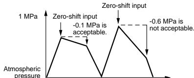
**Note 1:** The zero-shift function cannot be used in auto-tuning mode.
