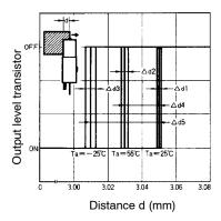
No. of repetitions: 20 at  $V_{cc}$  = 12 V
