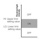
Set the value so that the upper limit setting value is larger than the lower limit setting value.
