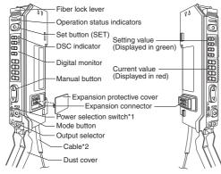
\*1 When set to "M", the power mode is fixed to Mega Turbo \*2 FS-V30 does not have the cable. M8 connector for FS-V31C(P)/32C(P)
