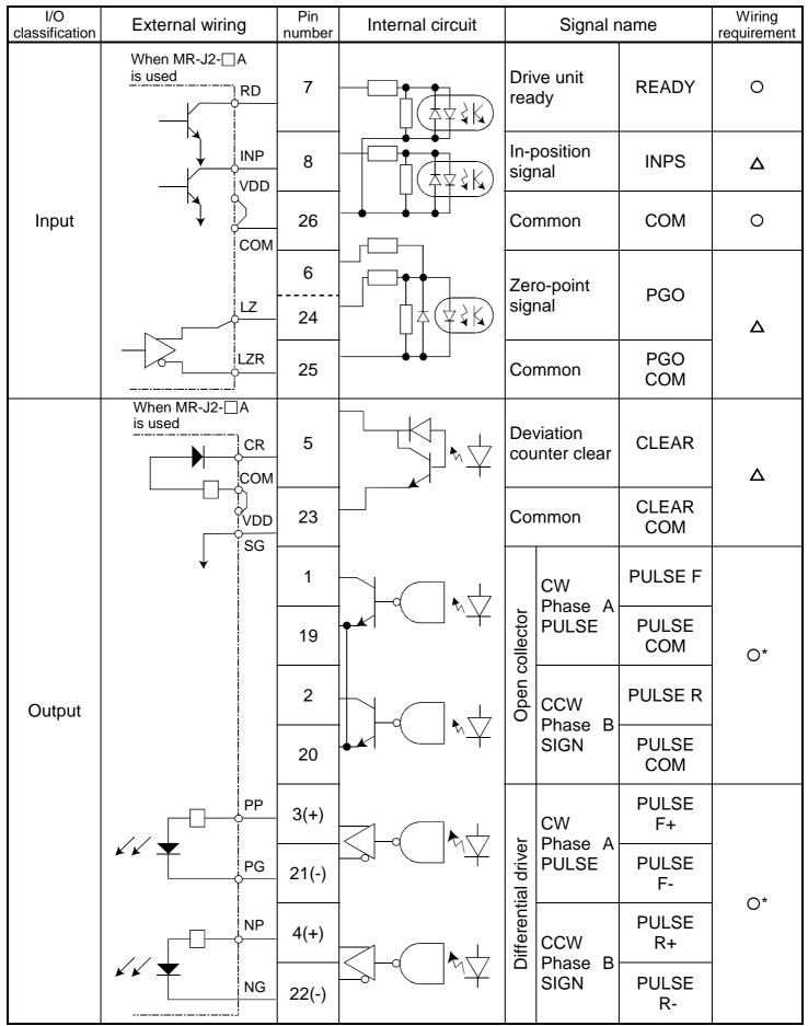
Select open collector output or differential driver output, according to the drive unit used.
