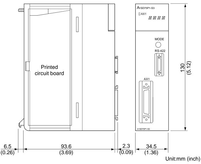
\* External dimensions are the same for A1SD75P1-S3, P2-S3 and P3-S3.
