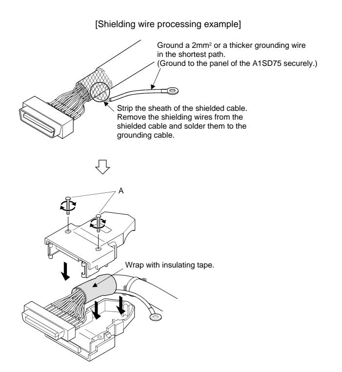
(11)To comply with EMC and low-voltage directives, use shielded cables and AD75CK cable clamp (made by Mitsubishi Electric) to ground to the panel.
